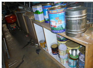
Poor storage of flammable liquids.
